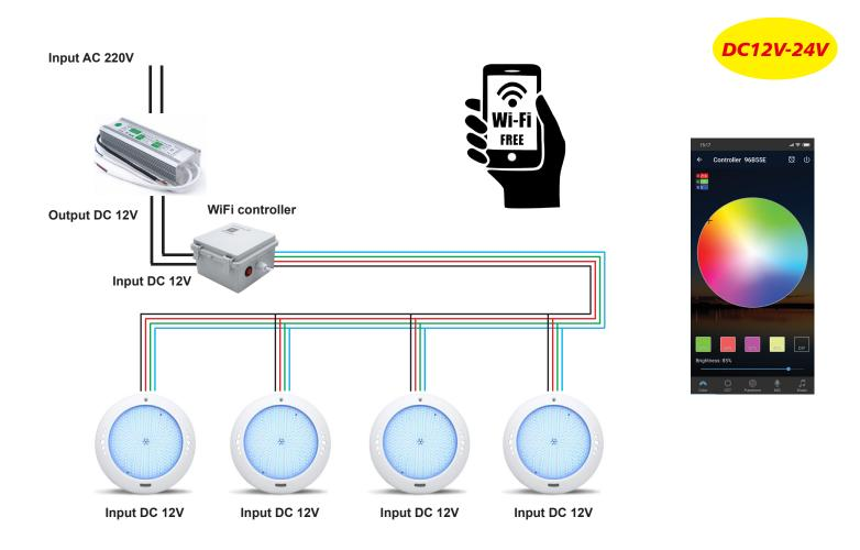
The RGB lights which connected with the Wifi CB004 box must be 4 wires, DC12V
